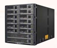
The E9000 chassis is 12 U high and features an optimized layout structure to maximally use space. It provides 16 slots and redundant power supply modules (PSMs), heat dissipation modules, management modules, and switch modules. The E9000 chassis can be installed in a standard 19-inch rack at a depth of at least 1,000 mm. Two types of E9000 chassis are provided: AC and DC.
